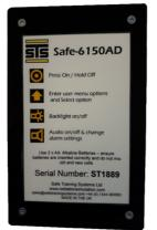
The simulator features the same display set out, audio output and button arrangements as the real
